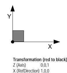
Local coordinate system for IfcBuildingStorey
