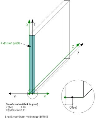
Local coordinate system for IfcWall Local coordinate system for IfcExtrudedSegment
