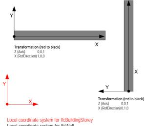
Local coordinate system for IfcWall
