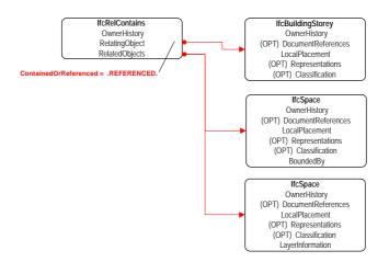
The same relationship types as for containment apply also for referencing containment. Each object can have only one IfcRelContains (of type .REFERENCED.), all objects that are referenced by the object must be referenced through the same IfcRelContains instance. The rules for referencing containment are a bit more relaxed in that the structure does not have to be hierarchical.
