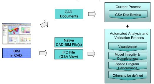
Version 1 of this BIM View is primarily focused on analysis of design performance relative to the GSA space program given to the architect at the outset of the project. While geometry and basic information is required for a primary set of building elements, emphasis has been put on properties of building spaces.
